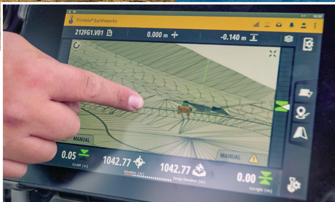
Top: Kon Construction's D6N with grade control and 3D GPS.
