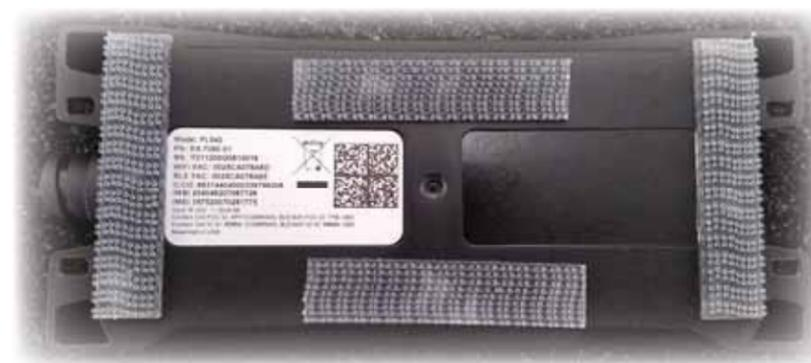
\*Use Dual Lock in the pattern above to mount the device.
