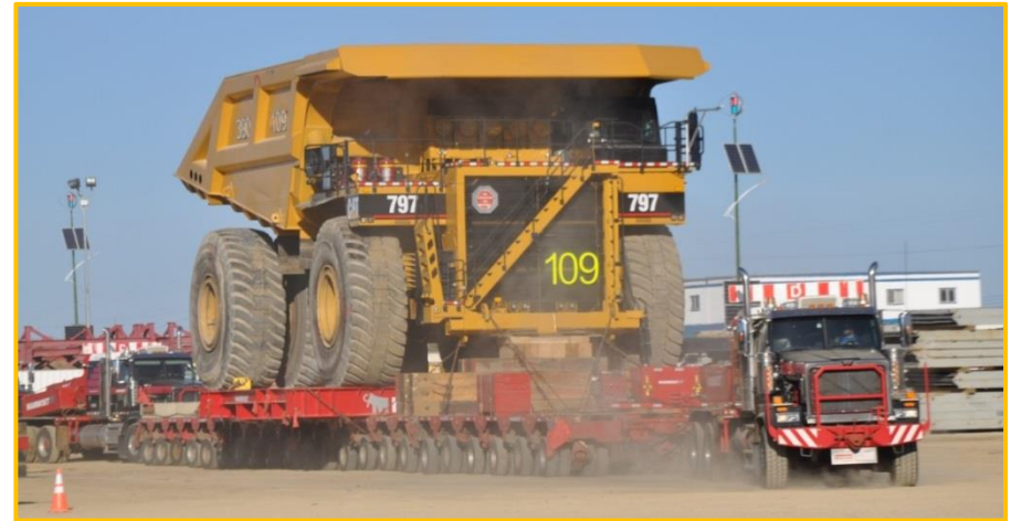
Hauling 797s to and from customer sites in one piece allows for maintenance and overhaul without site disassembly and return of trucks to customers mine-ready
