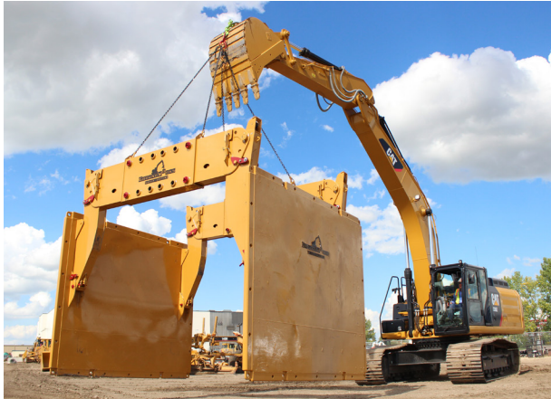
Finning offers items such as air compressors, pumps, lifts and trench shoring products (pictured) because customers ask for them.
