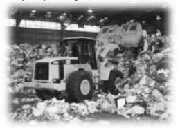
recycling centers and waste-to-energy plants. These arrangements provide value-added features that protect machine components, reduce debris entry and allow fast and easy cleaning. Added guarding is included for the radiator, windshield, power train, drive shaft, crankcase and front lights.
