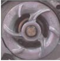
Cat® DEAC™ protected this water pump and earned a nine out of ten on the test.
