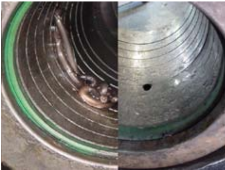
Cat® Hydraulic Hammer Paste provides a layer of protection between the tool and guide bushings.
