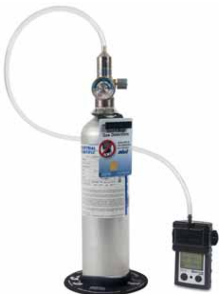
Diffusion monitor with positive flow regulator.
