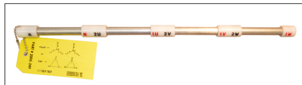
Shown above, 1:1 test jig, cat. no. 2005-249
