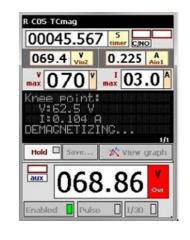
The Hand Held Control Unit, Raptor-HH, is the user-friendly interface from which the operator remotely control and monitor all the test process. This unit only weights 0,4 Kg and thanks to the TFT display, Touch Panel with Stylus, the Wheel
