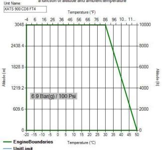
Graph represents working conditions, for starting conditions pls contact your Atlas Copco contact
