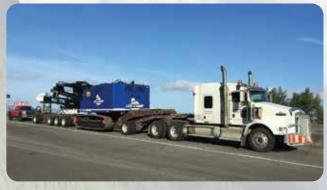
Easy relocation with a self folding boom and gantry, power tilting cab on both models. In addition the 550 can be moved in a single load.
