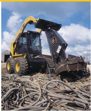
The S305 Mobile Scrap and Demolition Shear, mounted on a miniexcavator or skid steer loader is a very productive tool in processing of lighter steel or non-ferrous material such as cable, rebar, small beams and small diameter pipe.
