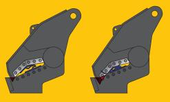
**Straight lower jaw enhances performance** – Maximizes shear force, creates a more efficient cut.
