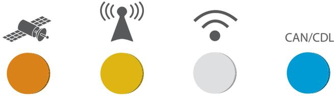
**ORANGE LIGHT:** This light should remain solid within a few minutes of installation. This indicates that the device has received a good GPS signal.
